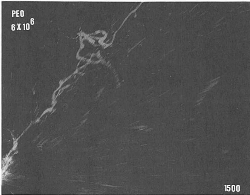
Figure 4. Spray cobwebbing behavior of PEO, 0.15 wt % aqueous solution.
